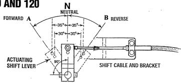
A greater amount of shift lever travel is in no way detrimental and is recommended. However, if the lever travel is shorter, proper clutch engagement might be impeded which, in turn, would mean premature wear, excessive heat generation and clutch plate failure. This would be indicated by slow clutch engagement or no engagement at all.
