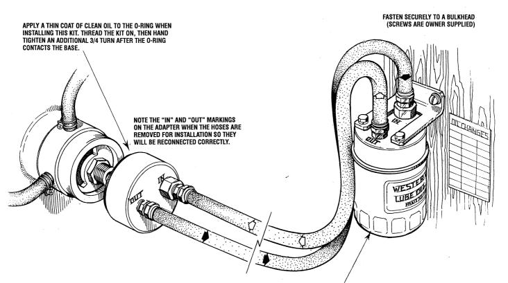
APPLY A THIN COAT OF CLEAN OIL TO THE FIL-TER GASKET WHEN INSTALLING. AFTER THE FILTER CONTACTS THE BASE, TIGHTEN IT AN ADDITIONAL 3/4 TURN.
