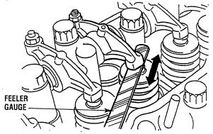
4. Loosen the lock nut for the adjusting screw. With a feeler gauge inserted between the rocker arm and valve cap, adjust the valve clearance by turning the adjusting screw. Make certain to adjust all the valves.
