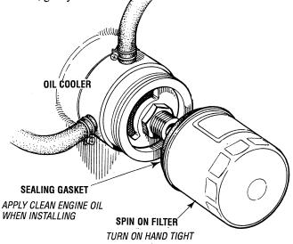
When installing the new oil filter element, wipe the filter gasket's sealing surface on the bracket free of oil and apply a thin coat of clean engine oil to the rubber gasket on the new oil filter. Screw the filter onto the threaded oil filter nipple on the oil filter bracket, and then tighten the filter firmly by hand.
