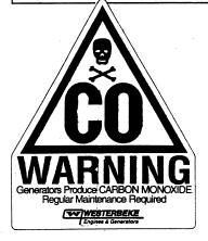
A WARNING DECAL is provided by WESTERBEKE and should be fixed to a bulkhead near your engine or generator.
