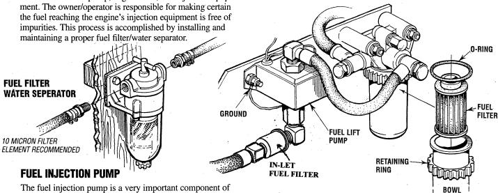
The fuel injection pump is a very important component of the diesel engine, requiring the utmost care in handling. The fuel injection pump has been thoroughly bench-tested and the owner-operator is cautioned not to attempt to service it. If it requires servicing, remove it and take it to an authorized fuel injection pump service facility. Do not attempt to disassemble and repair it.
