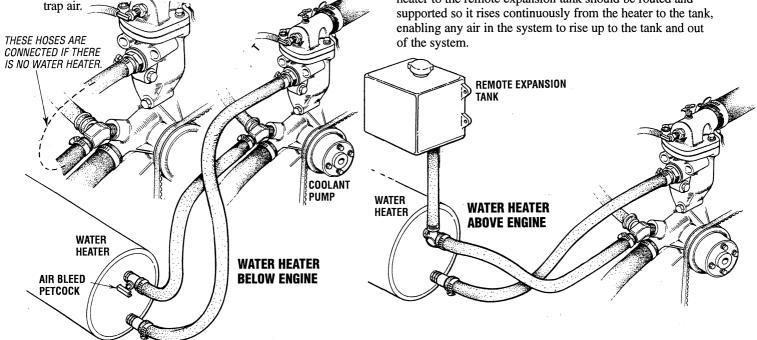
Hoses should rise continuously from their low point at the heater to the engine so that air will rise naturally from the heater to the engine. If trapped air is able to rise to the heater, then an air bleed petcock must be installed at the higher fitting on the heater for bleeding air while filling the system.
