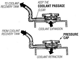
**NOTE:** Periodically check the condition of the manifold pressure cap. Ensure the upper and lower rubber seals are in
