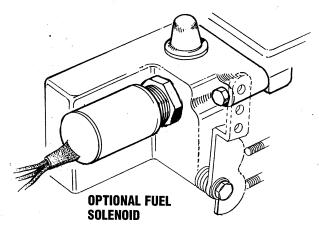
**NOTE:** Should the engine fail to shutdown when the key switch is turned off (goes to very slow idle), loosen the fuel solenoid's jam nut and screw the solenoid in 1/4 to 1/2 turn until shutdown is achieved.
