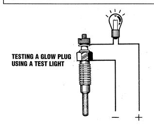
Re-install the plugs in the engine and test them again. The plugs should get very hot (at the terminal end) within 7 to 15 seconds. If the plugs don't heat up quickly, check for a short circuit. When reinstalling the glow plugs, use anti-seize compound on the threads.
